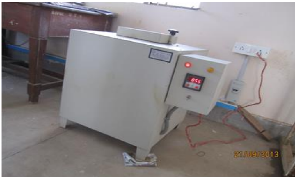
Figure 2.1 Pot furnace, with a stirrer
