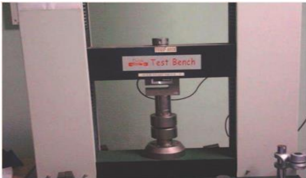
Figure 2-6 Experimental setup of compression test machine
